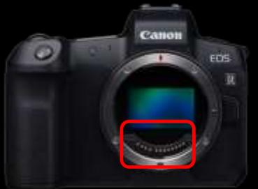
The EOS R system uses 12-pin electronic contacts to provide significantly improved communication between the camera and lens. Information such as the focus, zoom, aperture, and IS is instantly transmitted to the camera.
