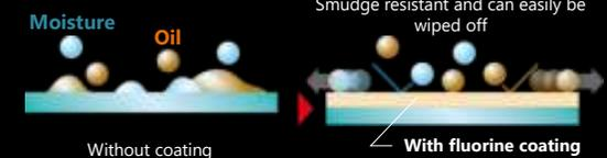
Fluorine coating is used on the front most and rearmost lens surface, making it easy to wipe off any oil from the lens with a dry cloth.
